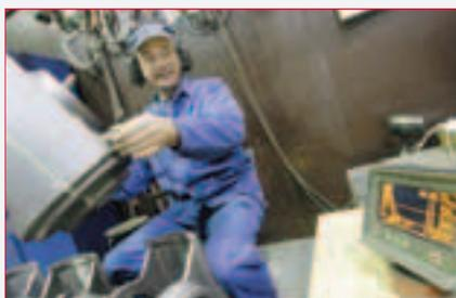
Componenta is committed to the continuous improvement of quality in all its operations. Quality control in production is continuous and different methods are used to ensure that cast products are defect-free. Mauno Kauppila uses ultrasonic testing to check that a cast component has no internal defects.
