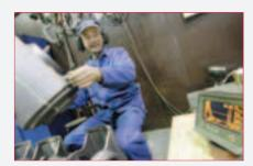
Componenta is committed to the continuous improvement of quality in all its operations. Quality control in production is continuous and different methods are used to ensure that cast products are defect-free. Mauno Kauppila uses ultrasonic testing to check that a cast component has no internal defects.
