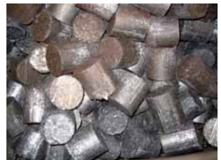
The machining chips compressed to form briquettes are remelted at the Pietarsaari and Orhangazi foundries.
